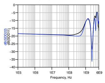
Figure 4. Differential Return Loss vs. Frequency (Zdiff=100  $\Omega$ )
