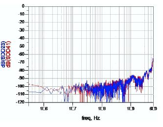
Figure 5. Differential Inter-Lane Cross-Coupling
