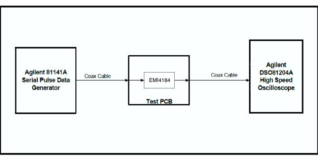
Figure 9. EMI4184 Eye Diagram Test Setup
