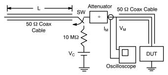
Figure 11. Simplified Schematic of a Typical TLP System
