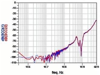
Figure 6. Common Mode Inter-Lane Cross-Coupling
