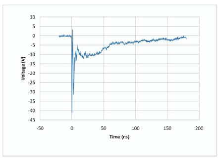
Figure 17. ESD Clamping Voltage -8 kV per IEC6100-4-2 (external to internal pin)
