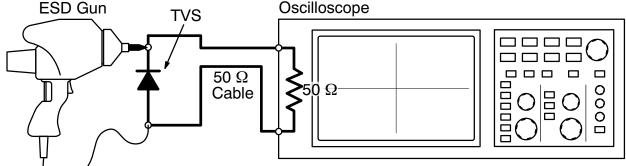
Figure 14. Diagram of ESD Test Setup
