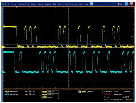
Figure 8. EMI4184 MIPI D-PHY LP Mode Measured Results
