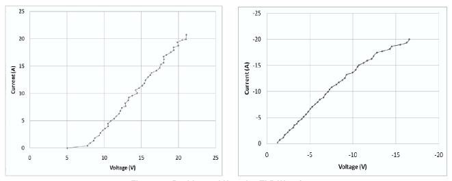
Figure 13. Positive and Negative TLP Waveforms
